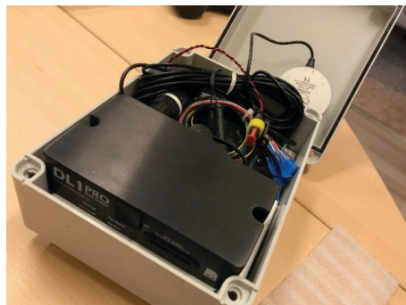
Figure 1: Demonstration of the secured case with DL-1 MK2 Data logger, GPS antenna and additional connector for output connections.
