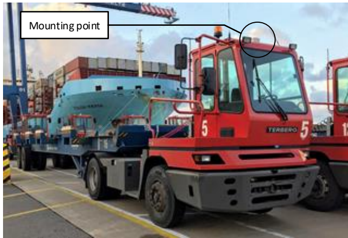
Figure 30. Demonstration of the trucks being used and the mounting point chosen for the experiments.
