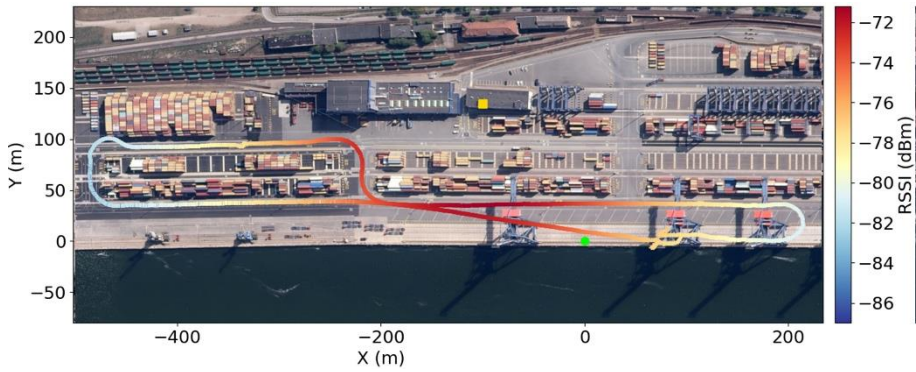
Figure 56. Visualization of experimental results of signal strength.
