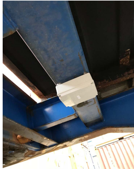
Fig. 5. Placement of the monitoring device under the truck due to constant physical contacts that could potentially cause damage to the equipment.
